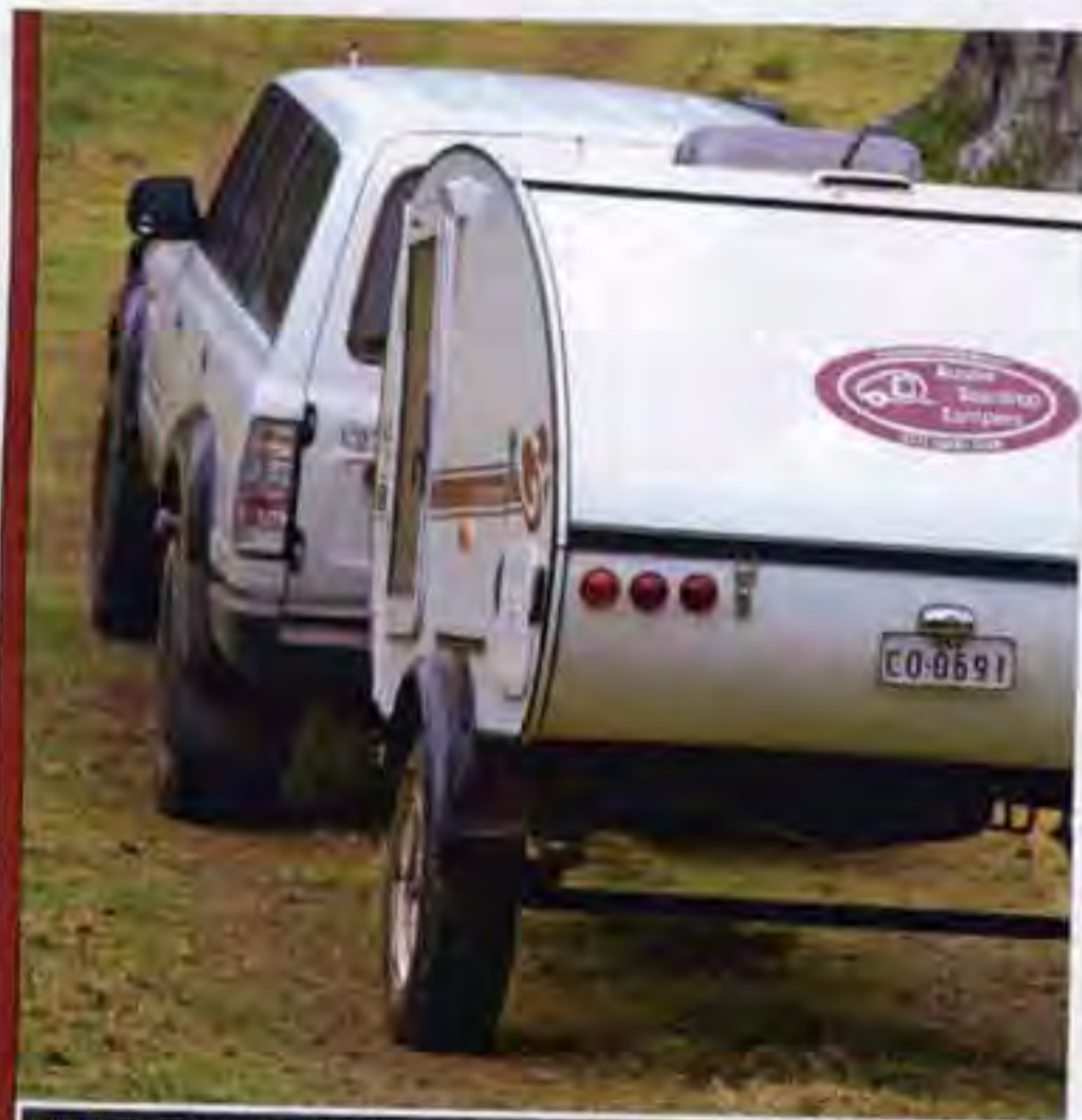
The Adventuretear is the 'heavy off-road' model in Aussie Teardrop's range, if you can call anything that weighs 560kg 'heavy', and with 15in eight-ply tyres and 'spring over' leaf packs it has all the ground clearance you need for anything short of severe off-road conditions
