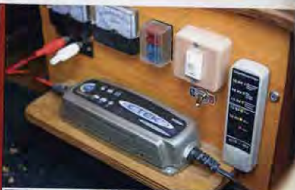
Electrics are very simple and easy to monitor too. The battery is charged by a smart charger that can be switched to power mode if you're hooked to shore power. It'll run for days powering the lights and stereo, and there's no doubt about when you'll need to charge it either.
