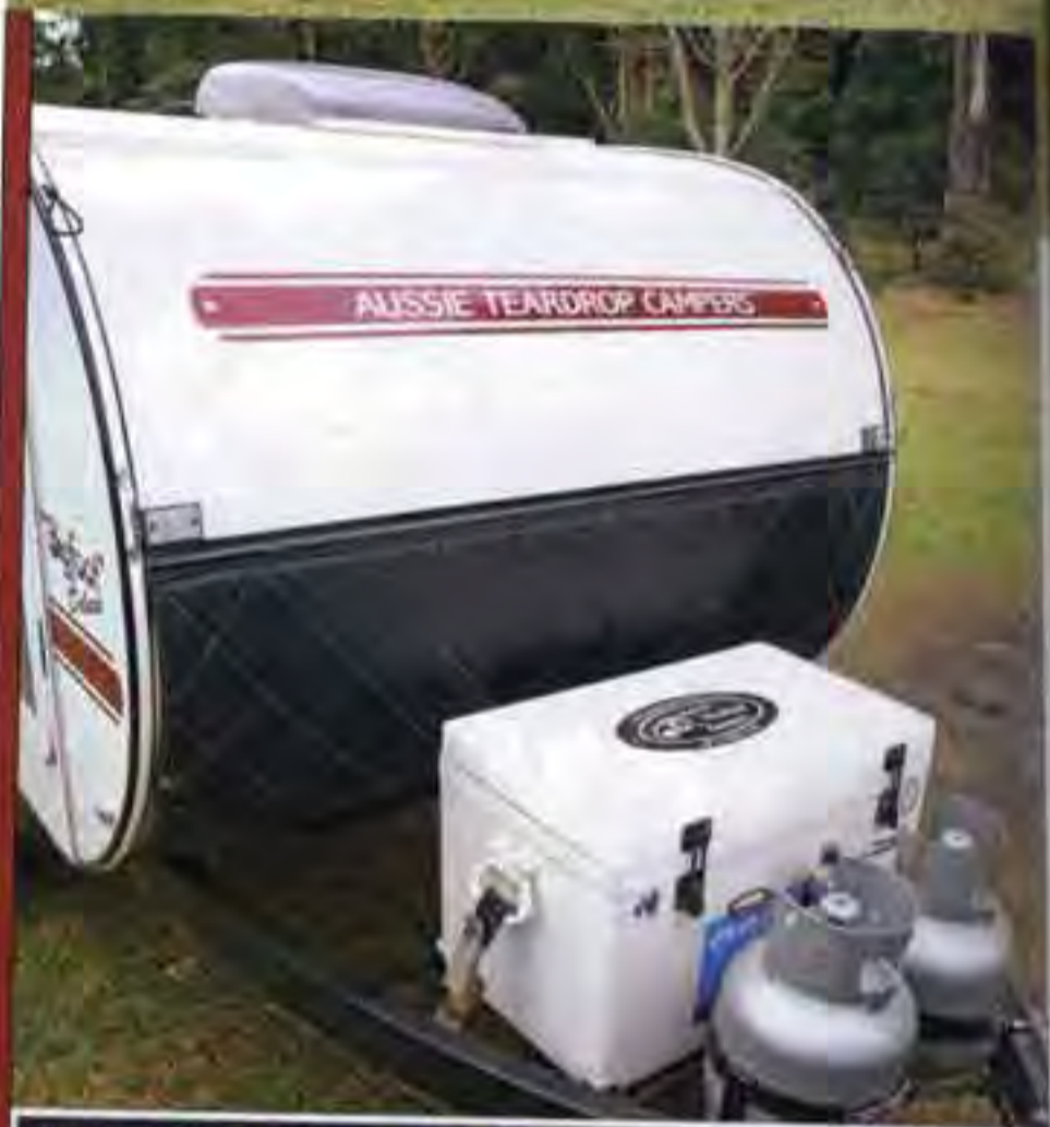
A huge icebox and two 4.5kg LPG bottles are standard equipment, but no doubt you could opt for a fridge if the mood took you. I used the truck fridge and kept the esky full of ice – and refreshments! Note the 100x50mm A-frame – overkill engineering at this weight!
